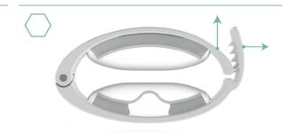
Open the clamp by pulling the retention and lifting the upper part.
