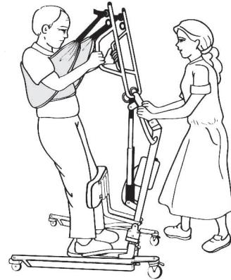
**⚠ WARNING: Do not lock or block the patient lift casters when lifting. The casters must be free to roll so that the patient lift can stabilize as the patient is lifted from the bed.**
