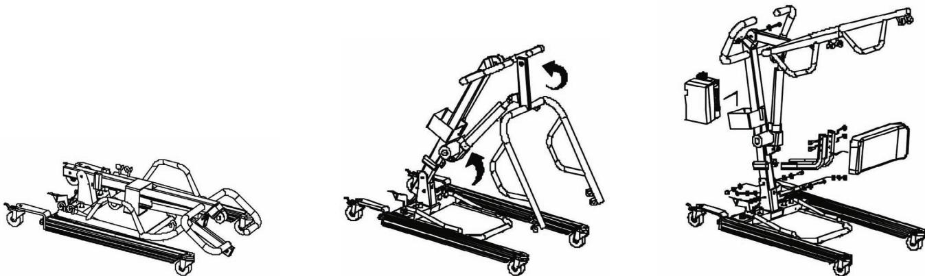
1. Remove the nuts and bolts from top and bottom of mast.
